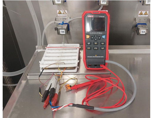
Fig. 7. Showing the UT622E, connected to the plate capacitor setup.
